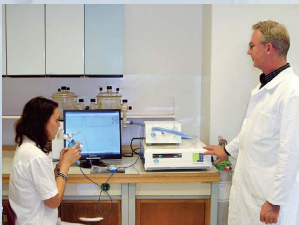
Detection of exhaled nitric oxide using a chemiluminescence analyzer
